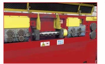
Two infeed units drive properly the wire, guaranteeing constant speed and straightening quality, making it particularly suited for small diameters. Based on the different lengths and diameters can be possible to work with setting of different speeds.
