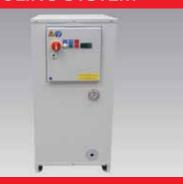
• The machine electrical motors and other devices, such as the control panel, are cooled through a forced liquid cooling system. For this purpose a refrigerating unit is used to keep the liquid at the set temperature.
