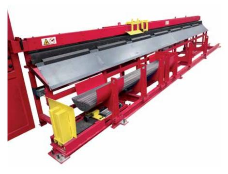
The guiding support available in several versions, allowing the collection and distribution of straightened bars according to the specific production needs.
